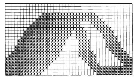
The actual pattern **that** the printer prints on **the** paper is made up of dots that overlap each other both vertically and horizontally. The reason the planning grid uses  $an \times for each$  dot is that using an accurate representation of **the** dots makes calculating the data numbers difficult because they cover each other. Therefore, remember that  $each \times for each = for eac$
